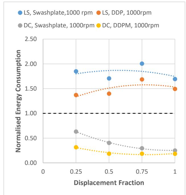
**FIGURE 9: 95 BAR, 1000RPM SIMULATION RESULTS.**
