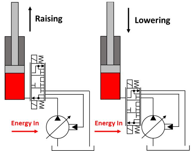
**FIGURE 9: SIMPLIFIED CIRCUIT SCHEMATIC OF CONVENTIONAL LOAD SENSE PUMP RAISING AND LOWERING A BOOM.**
