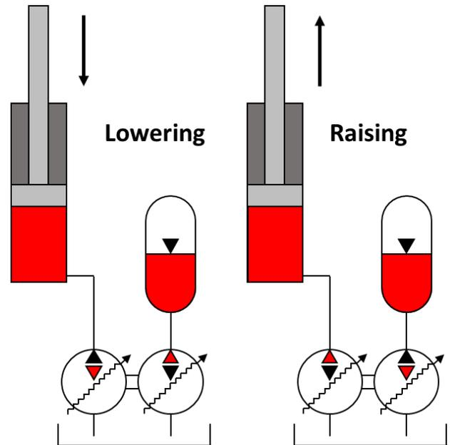
**FIGURE 2:** SIMPLIFIED SCHEMATIC OF TRANSFORMING TO AND FROM AN ACCUMULATOR WITH A MULTI SERVICE DDPM.
