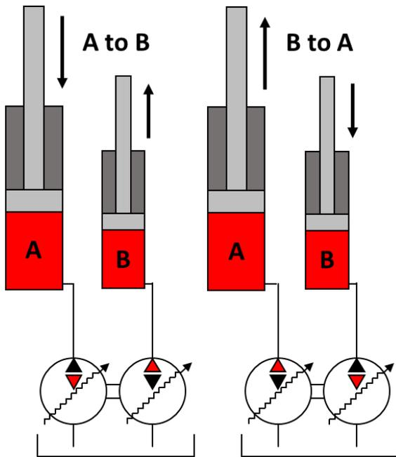
**FIGURE 1:** SIMPLIFIED SCHEMATIC OF TRANSFORMING BETWEEN ACTUATORS WITH A MULTI SERVICE DDPM.
